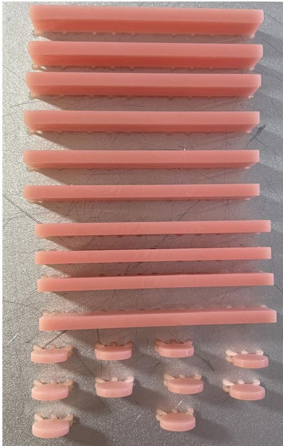
**Fig. 3** Denture base resin specimens modified with 1wt% cerium oxide nanoparticles
