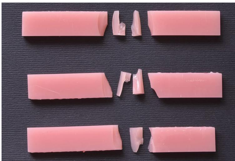
**Fig. 5** Flexural strength specimens after fracture
