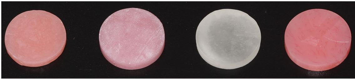
**Fig. 1** One representative specimen fabricated by injection molding, 3D printing, conventional heat-polymerization and milling technique, respectively
