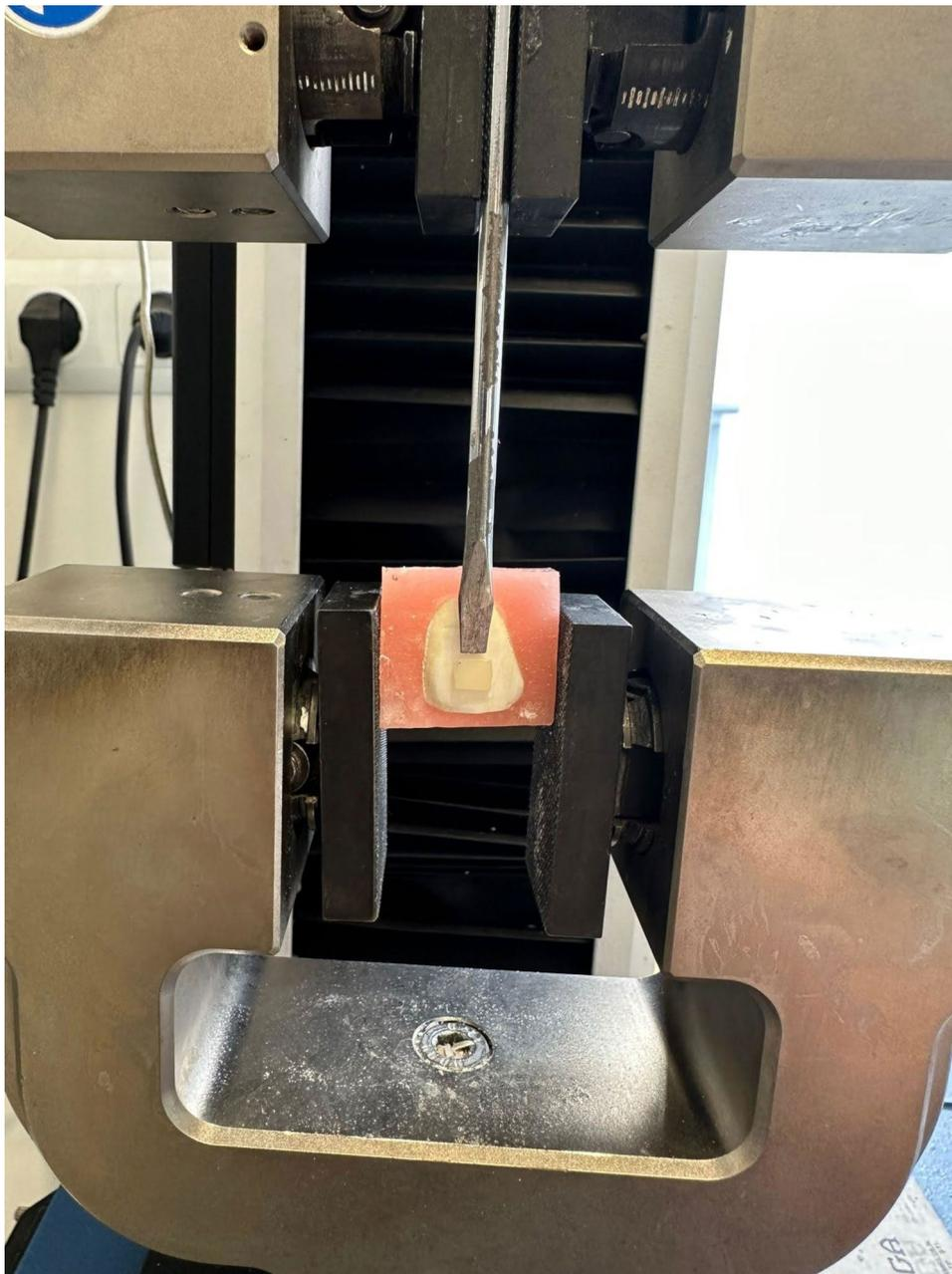
**Fig. 1** A photographic illustration of the shear bond strength test being conducted using an Instron machine
