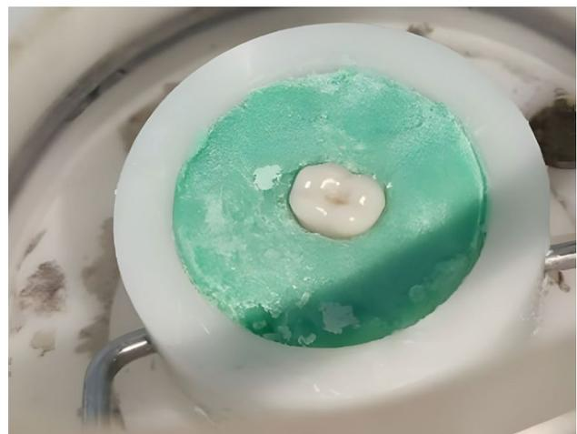
**Fig. 2** Conventional tooth specimen secured in the middle of its holder using auto-polymerizing resin
