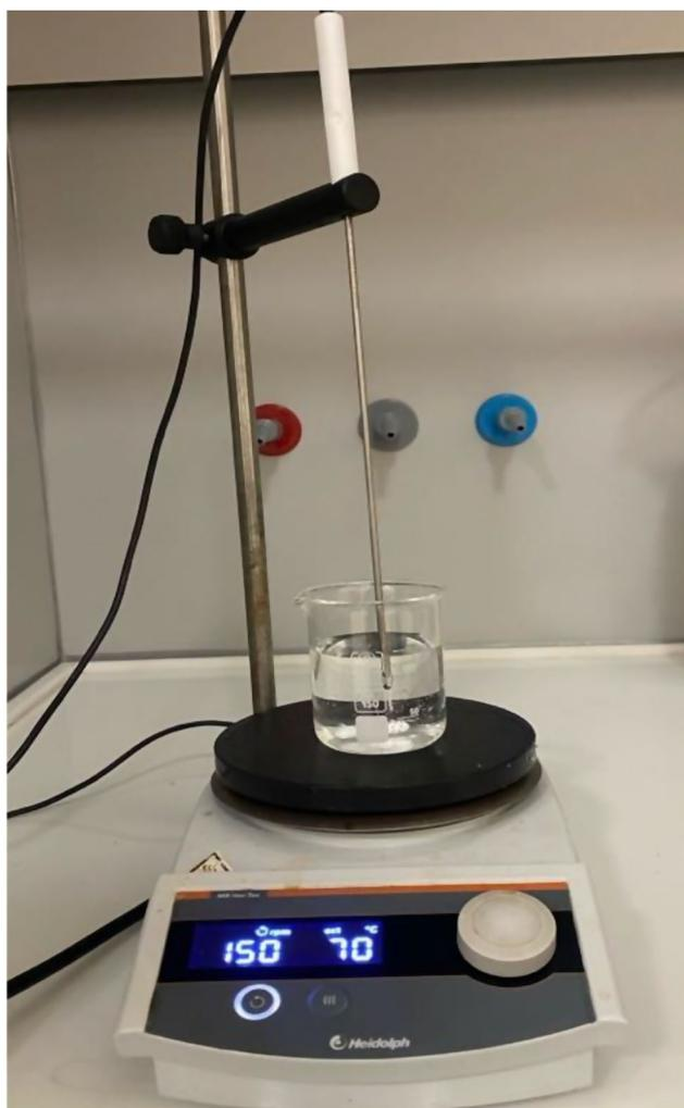
**Fig. 1** Sodium hypochlorite solution being heated using a digital hot plate magnetic stirrer device (Heidolph MR Hei-Tec)
