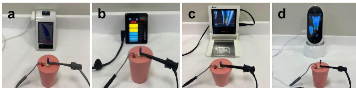
**Fig. 2** The experimental setups used in measurements with EALs are as follows: **a**;Root ZX Mini, **b**;Propex Pixi, **c**;Raypex 6, **d**;Ai-Pex
